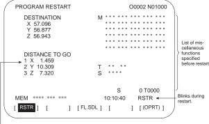
Axis sequence set in parameter No. 7310 (Displays \* when the preparation for restart is not completed. Displays the axis sequence when searching the restarting block is completed. Blinks when the preparation is completed.)
