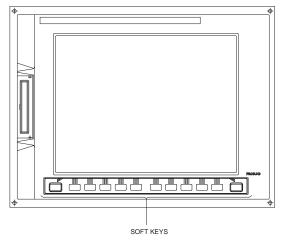
Fig.1.1 (b) CNC Control Unit with 9.5"/10.4" LCD
