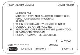
2 Press soft key [(OPRT)], enter the alarm number, and then press soft key [SELECT] to display the help message for the alarm corresponding to the entered number.
