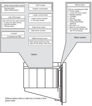
On a unit with two option slots, two option boards can be mounted.
