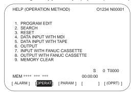
Press soft key [(OPRT)], enter the number of the item to be displayed, and then press soft key [SELECT] to display the operation method.
