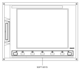
Fig.1.1 (a) CNC Control Unit with 7.2"/8.4" LCD
