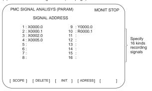
(a) [SCOPE] soft key : Select the signal wave display screen.
