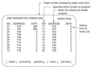
Setting time : Timer No. 1-8 =Max.=1572.8 sec, each 48msec. Up to 262.1 seconds in units of 8 ms for timer Nos. 9 to 40 subsequent timers (timer Nos. 9 to 150 in the RB6/RC4)
