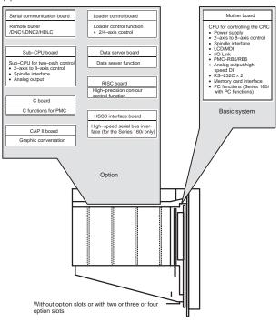
On a unit with two option slots, two option boards can be mounted. On a unit with three option slots, three option boards can be mounted. On a unit with four option slots, four option boards can be mounted. (On the unit with four option slots, just a data server board or HSSB interface board can be fit into the slot furthest from the LCD.)
