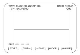
4 Press the [START] soft key. In the upper part of the screen, the word SAMPLING blinks, indicating that data sampling has started. Upon the completion of data collection, a waveform is displayed automatically.
