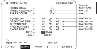
Not counted when the option for displaying the operation time and  $\,$  – the number of parts is not provided.
