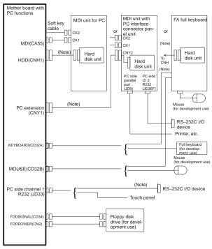
NOTE The cables for the hard disk unit, PC interface connector unit and FA full keyboard are provided by FANUC.
